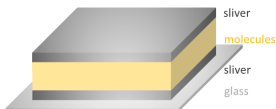
Figure 3.3. Diagram of the sandwich structure molecules in optical cavity.
